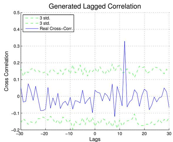
FIG. 4: The cross-correlation sequence two generated time series. Time series  $y_1(t)$  was generated by a poisson random number generator while  $y_2$  is a linear combination of values of  $y_1(t - 12)$  and white noise. The blue (solid) line represents the actual cross-correlation sequence while the green (dotted) lines represent  $3\sigma$  intervals from a null model created by randomly permuting the time series and calculating the a distribution of cross-correlation series.
